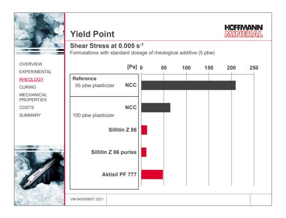
If the yield point is to bring back to the level of the reference formulation (with 55 pbw plasticizer), when working with Sillitin – as illustrated in the figure for Sillitin Z 86 puriss – about 11 pbw rheological additive are required, and with the hydrophobically treated grade Aktisil PF 777 about 9 pbw.
