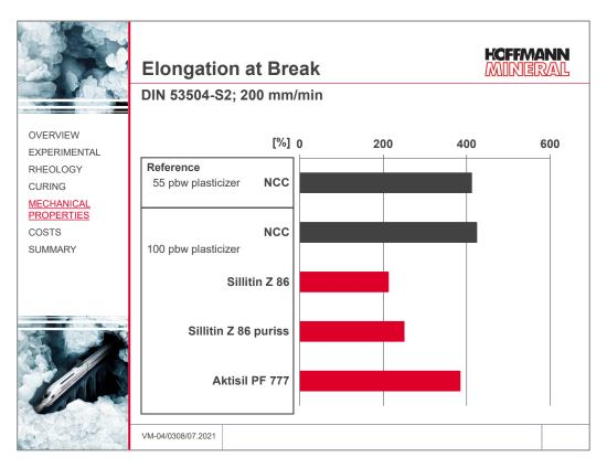
Up to 50 % elongation, also Neuburg Siliceous Earth gives low tensile moduli, while with Aktisil PF 777 the stress/strain ratio at 100 % elongation remains comparable.
