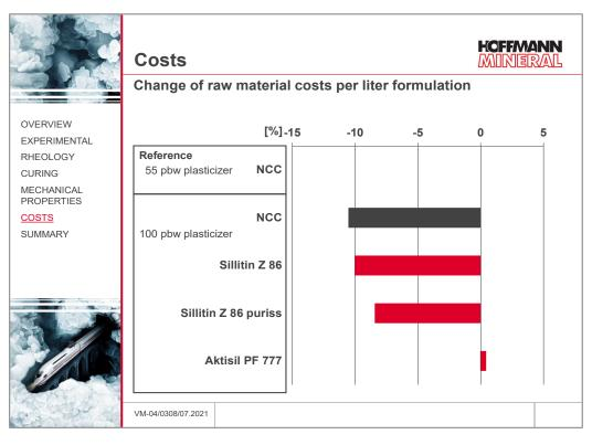
Even with an adjusted yield point and therefore higher raw material costs for the rheological additive, the costs per formulation with Sillitin remain below the level of the reference. Aktisil PF 777 gives rise to a slight cost increase.
