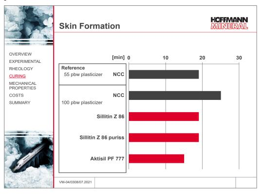
For the assessment of full cure, the extrudate was cut open after different periods of time, and the thickness of the cured layer was determined with the aid of a caliper rule.
