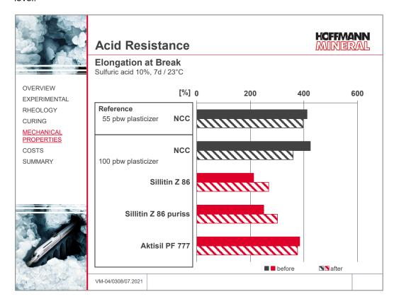
These effects come out particularly distinctly when comparing the percentage changes: the acid exposure of the untreated siliceous earth grades Sillitin Z 86 and Sillitin Z 86 puriss causes a similar loss of the tensile strength as with the calcium carbonate formulation, but elongation at break increases with the siliceous earth filler. Aktisil PF 777 with respect to tensile strength and elongation remains much more resistant than the other fillers.
