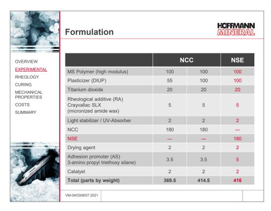
Starting from the base formulation with 180 parts by weight (pbw) of natural calcium carbonate and 55 pbw plasticizer, the loading of Neuburg Siliceous Earth and plasticizer was to be adjusted in a way to arrive at comparable tensile moduli in the tensile test. For Neuburg Siliceous Earth, this could be achieved with 100 pbw of plasticizer along with 180 pbw of filler.
