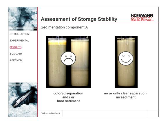
The samples were stored for 10 weeks at 40 °C, which would correspond in actual fact to a storage time of 18 months at room temperature. With the systems tested, differences were only observed with respect to the amount of clear supernatant liquid, while no sediment was formed in any case. With the same additives, Neuburg Siliceous Earth imparts less tendency towards separation than barite. The largest amount of separation was found for the fine filler free formulation.
