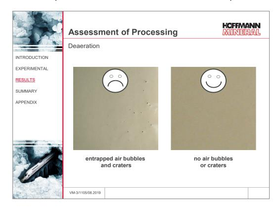
Shortcomings are particularly evident with the treated silica formulations. The largest differences come out in the additive-free systems. The barite/silica combination, in contrast to Sillitin Z 86, here leads by far to the poorest deaeration performance.
