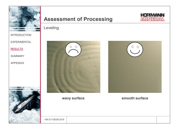
On principle, the compounds with the barite/treated silica blend offer slight advantages in leveling because of the lower volume filler proportion. When eliminating the additives, how-ever, the leveling properties heavily change in favor of the Sillitin Z 86 batch.
