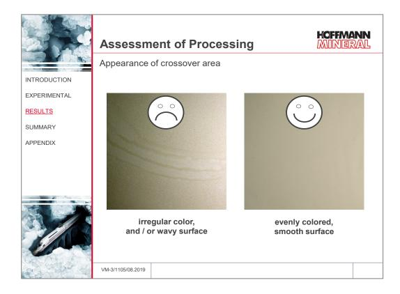
The visible transition of adjacent, subsequent batches is more pronounced, even after working with the spiked roller, for the barite compared with the Sillitin formulations. The best results were obtained with the additive-free Sillitin Z 86 compound, where no color or structure changes could be observed in the crossover area.
