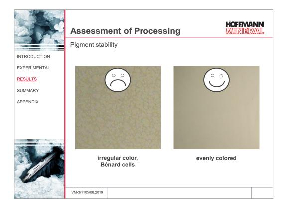
The formulations containing Sillitin Z 86 offer a more "uniform" visual impression compared to the systems without filler resp. with barite.
