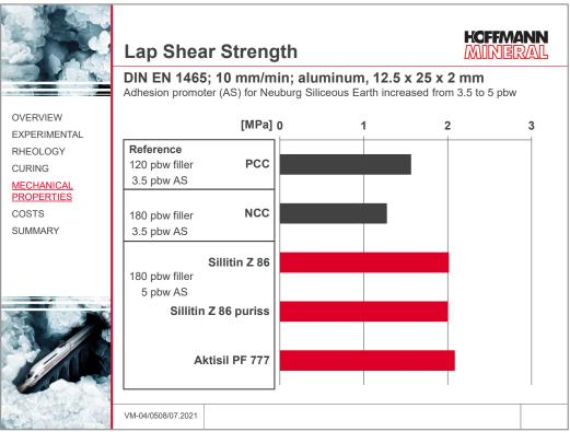
In order to assess the deformability of the adhesive joint, the shift distance was measured in the lap shear test. Neuburg Siliceous Earth here gives rise to a distinctly different stress/strain curve with a markedly reduced shift distance.
