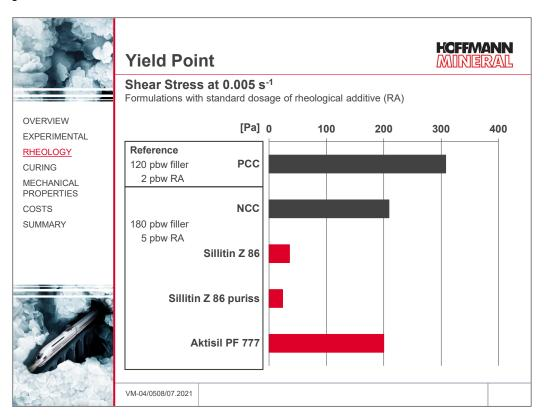
In order to adjust the yield point to the level of the reference formulation (precipitated calcium carbonate + 2 pbw rheological additive), working with Sillitin – here illustrated on the example of Sillitin Z 86 puriss – requires a dosing of 12 phr rheological additive. The hydrophobic grade Aktisil PF 777 needs approx. 7 pbw.
