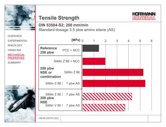
On the other hand, the high elongation at break of the calcium carbonate could not be attained with Neuburg Siliceous Earth. Between the two grades tested; Sillitin V 85 tends to give higher values.
