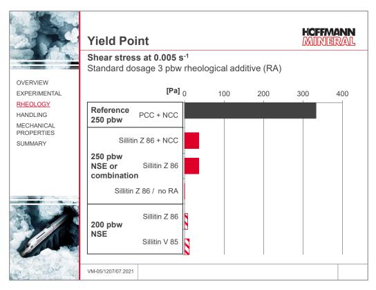
In a further test series, the concentration of the rheological additive was varied in order to affect the yield point. In view of the mentioned viscosity increase when replacing the calcium carbonate at equal weight, tests were only run with a reduced filler loading of 200 pbw.
