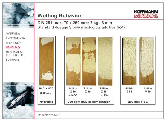
Even with the highest addition of the rheological additive (and the same yield point as the reference formulation), the batches with Neuburg Siliceous Earth give rise to markedly superior wetting.  $^3$
