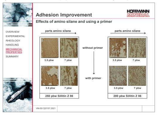
The very best results for the tensile shear strength were obtained with an increased dosing of the adhesion promoter in conjunction with the use of a primer.  $^{\rm 4}$
