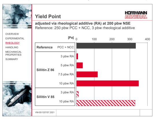
Along with the yield point, with higher additions of the rheological additive also the viscosity shows an increase, and this more so with Sillitin Z 86 with Sillitin V 85.
