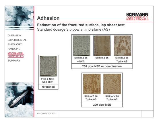
Although the fracture surfaces of the formulations with Neuburg Siliceous Earth, contrary to the reference formulation, do not give evidence of 100 % cohesive failure, these fillers all the same lead to a marked increase of the tensile shear strength.
