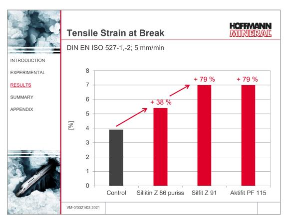
With Neuburg Siliceous Earth, a marked increase in tensile strain at break is obtained, especially with the two calcined grades. Silfit Z 91 and Aktifit PF 115 achieve an approx.
