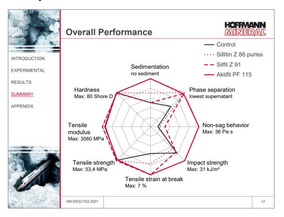
Neuburg Siliceous Earth is very well suited as a functional, mineral filler for heavy-duty 2K PU coatings.
