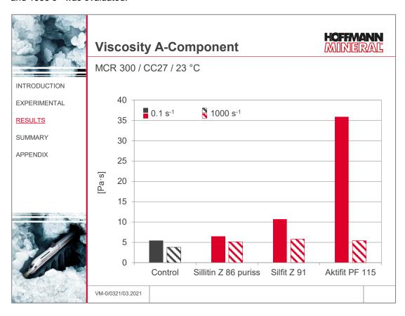
The high shear rate (shaded columns) represents the behavior during pumping processes as well as the behavior during application. Here, hardly any difference between the formulations is detectable.
