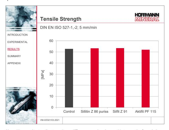
Also with regard to tensile strength, no difference can be observed between the formulations.
