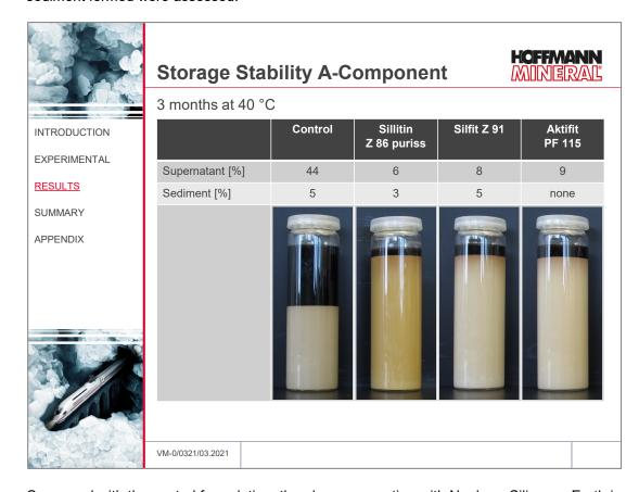
Compared with the control formulation, the phase separation with Neuburg Siliceous Earth is clearly reduced. As with the control formulation, however, also with Sillitin Z 86 puriss and Silfit Z 91 a relatively solid sediment is formed over the storage time. With Aktifit PF 115, sediment formation can be completely prevented. The formulation is thus much easier to homogenize and thus perfectly storage stable.
