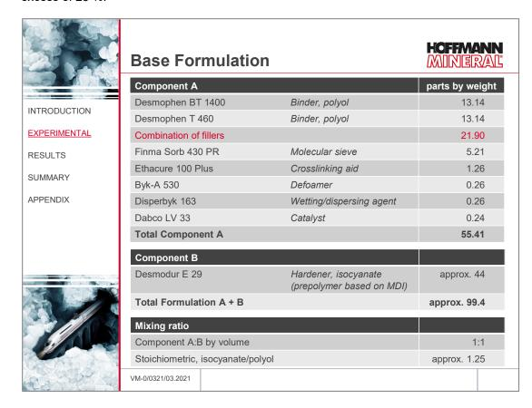
The filler combination in the base formulation consists of barite, a natural mica-chlorite-quartz intergrowth (leucophyllite) and a quartz flour surface treated with epoxy silane. In the tests, the leucophyllite and the quartz flour were replaced by products of Neuburg Siliceous Earth in equal weights. The barite remained present in all formulations and was dosed unchanged.
