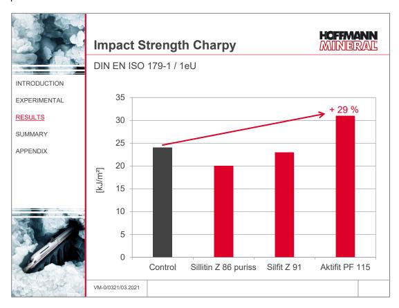
While the formulations with the non-surface treated Neuburg Siliceous Earth grades Sillitin Z 86 puriss and Silfit Z 91 are on a somewhat lower or comparable level as the control formulation, the impact strength with Aktifit PF 115 increases markedly by approx. 30 %.
