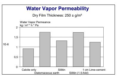
Using this method, water vapor permeability can easily calculated, as follows: kg (water vapor) / m<sup>2</sup> (sample surface area) - hours - Pa (water vapor partial pressure).
