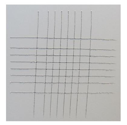
Test with tape tear-off [GT] Drying 7 d 23°C as well as + 7 d 50°C convection drier
