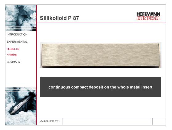
During the extrusion of 2.5 kg of the compound with Sillikolloid P 87 a continuous layer of deposit is formed on the total surface of the metal insert. At the end of the test, deposits are observed also on the total surface opposite the metal insert, which increase towards the exit region. Over the whole, markedly more deposit is found than with Sillitin N 85. The visual assessment at 100x magnification confirms these results.
