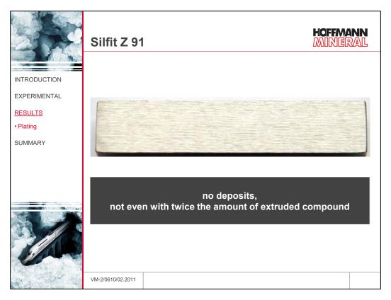
In contrast to the previously mentioned fillers even after extruding twice the amount (5 kg) of the compound with Silfit Z 91 neither with the naked eye nor at 100x magnification deposits are made out on the metal insert.
